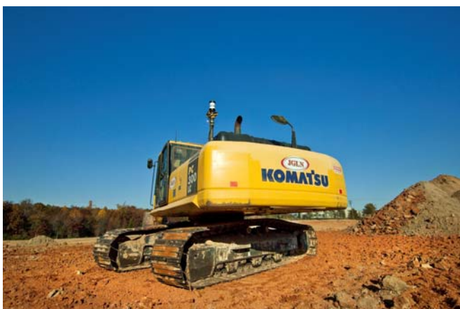
Graphic: Komatsu Excavator GCS900 with MT900 Machine Target.jpg
